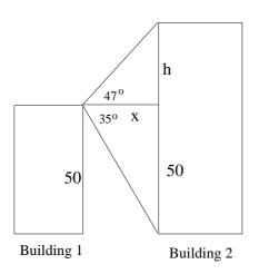
The diagram above shows the situation described in this problem. To find the total height of the second building, we first find the distance between the two buildings using the fact that  $\tan 35^\circ = \frac{x}{50}$ , therefore,  $x = \frac{50}{\tan 35^\circ} \approx 71.41$  feet.
