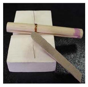
You see the complete motor making jig in the photo to the left. The  $\frac{1}{2}$  inch diameter dowel is tapered slightly to allow the wire to slip off easily. The dowel also has grooves in the sides 180 degrees apart to allow the wire tails to be easily wrapped around the loop.
