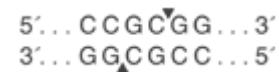
Figure 5. SacII cleaves the phosphate backbone of DNA between the C and G bases as shown, in any DNA which has its exact recognition sequence.
