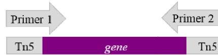
Figure 7. This diagram shows how specific primers are used to sequence a portion of the transposon DNA and the genomic DNA flanking either side to reveal the interrupted gene that caused the mutation. Primer sequences may be found in the appendix.
