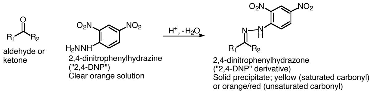
Put 4 pipets of 2,4-DNP solution into a large test tube, add a magnetic stir bar, and to a well-stirred solution add 30 drops of your unknown. After 5 minutes, cool, add 2 pipets of cold water, filter, wash with cold water, and wash with a small amount (three pipets) of cold ethanol. Aspirate thoroughly, and hopefully get a crude mp. Recrystallize (or "digest") from anhydrous ethanol, using a 125-mL Erlenmeyer.
