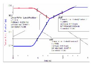
each end. For this experiment, in Logger *Pro* the direction of one detector was reversed, and then both detectors are zeroed with the carts stuck together near the middle of the track. This places the origin of the common coordinate system near the middle, and the two readings will then be the same when the carts are in contact.
