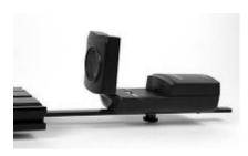
Newer Vernier Motion Detectors (green or black case with adjustable sensitivity) can be placed so that the sensor is 15 cm from the end of the track. The carts can then be detected properly all the way to the end. The track mode is appropriate for the dynamics system.
