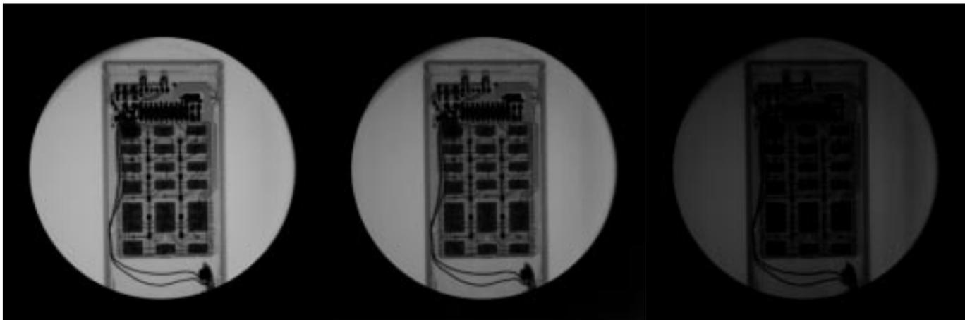
Fig. 2 Luminous-screen image of a pocket calculator (photographed using a digital camera) at maximum tube high voltages and different emission currents.
