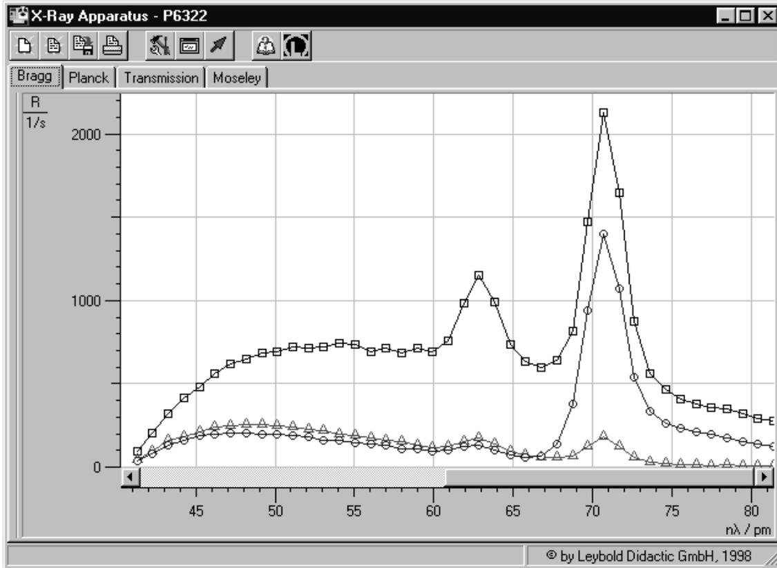
Fig. 4 Diffraction spectra of x-rays with ▲ the characteristic lines of the molybdenum anode in the wavelength range between 40 and 80 pm ( $U = 30$  kV)
