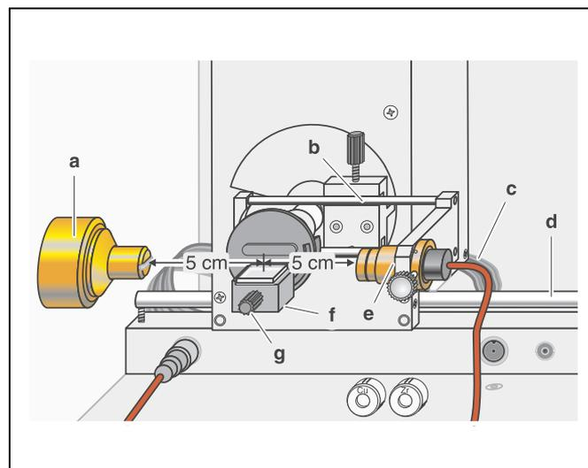
Fig. 3 Experiment for investigating the wavelength-dependency of the attenuation coefficient
