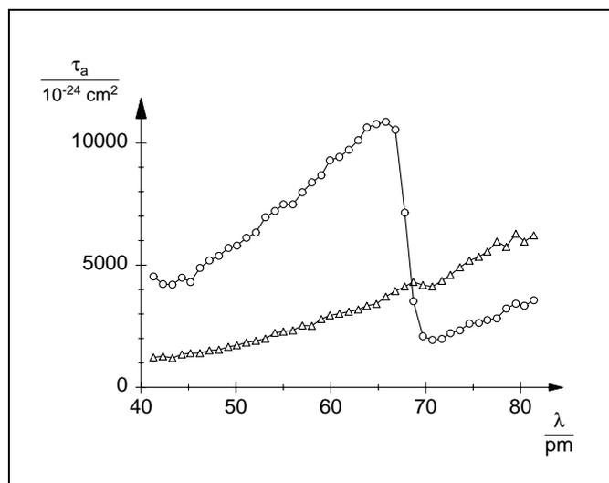
Fig. 7 Absorption cross-section  $\tau_a$  shows as  $\ln \tau_a$  as a function of  $\lambda$ .
