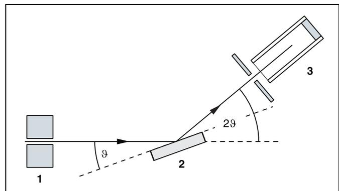
Fig. 2 Diffraction of x-rays at a monocrystal and for  $2\vartheta$  coupling between counter-tube angle and scattering angle (glancing angle)
