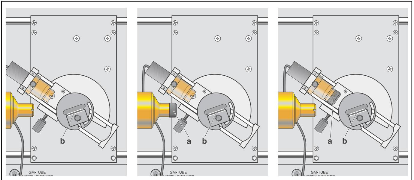
Fig. 3 Experiment setup for verifying the wavelength shift due to Compton scattering
