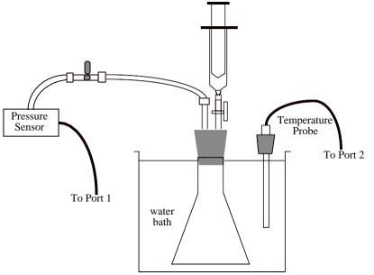
3. The live pressure reading at the bottom of the window should be the atmospheric pressure. Record the atmospheric pressure and the temperature values in your laboratory notebook.
