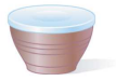
(b) Closed system: A cup of hot soup with a lid Mass constant
