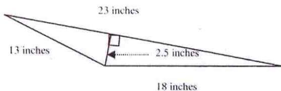
$$\begin{aligned} \text{Area}_{\text{triangle}} &= \frac{1}{2}bh = \frac{1}{2}(23)(2.5) \\ &= 28.75 \text{ in}^2 \end{aligned}$$
