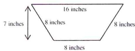
$$\begin{aligned} \text{Area}_{\text{Trap}} &= \frac{1}{2}(B+b)h \\ &= \frac{1}{2}(16+8)7 \\ &= 84 \text{ in}^2 \end{aligned}$$
