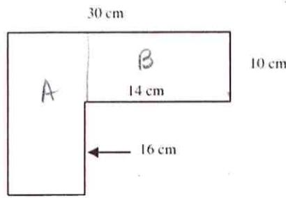
$$\begin{aligned} \text{Area} &= \text{Region A} + \text{Region B} \\ &= (16 \times 26) + (14 \times 10) \\ &= 416 + 140 = 556 \text{ cm}^2 \end{aligned}$$
