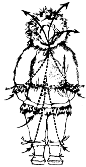
Figure 5.3 The Chimney Effect in Inuit Fur Clothing Vents in the clothing can be opened by release of drawstrings during exercise to prevent accumulation of sweat.
